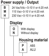
Example: CP302-BOA = pressure transmitter type CP 300, with measuring range of -500/+500 Pa, with power supply 24 Vac/Vdc, 0-10 V or 4-20 mA output, with display and alu housing.
