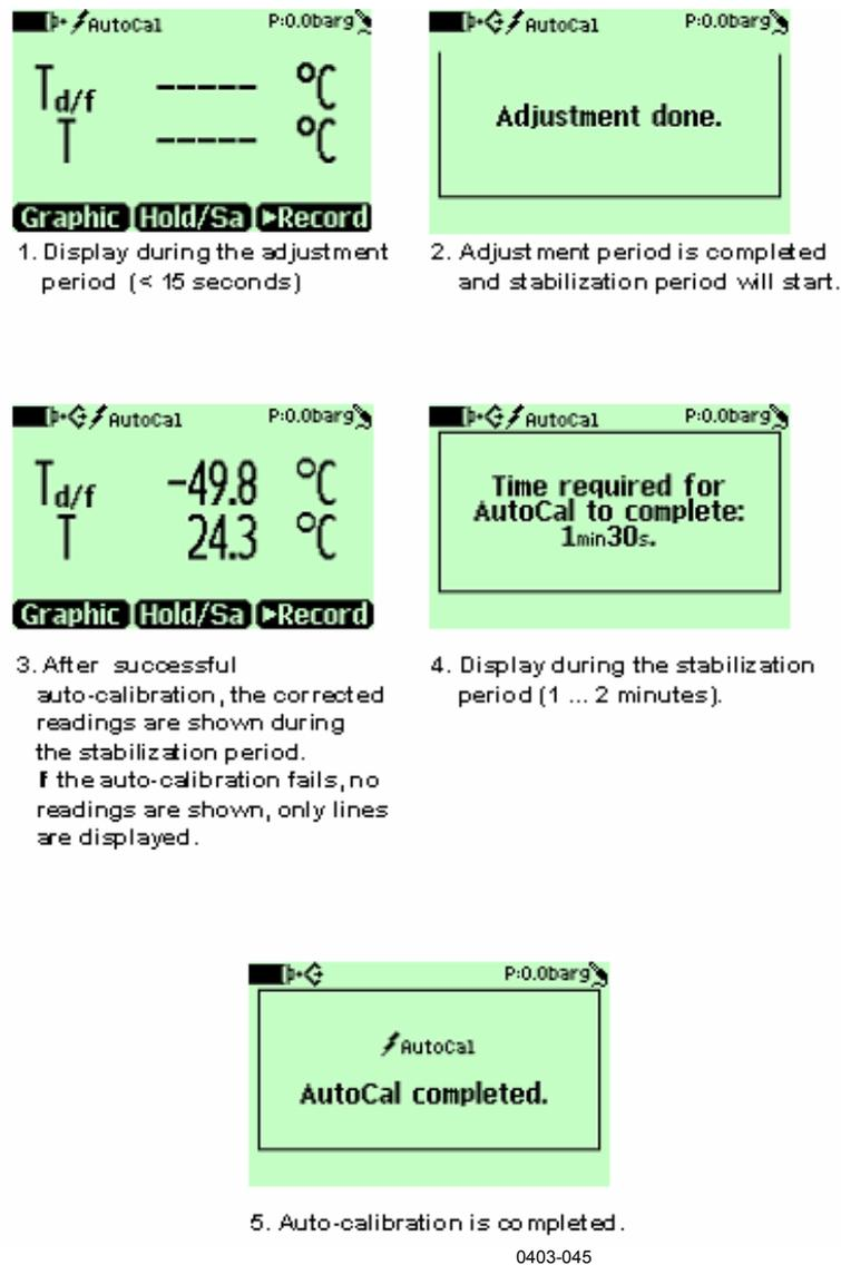
**Figure 9** Auto-Calibration Displays
