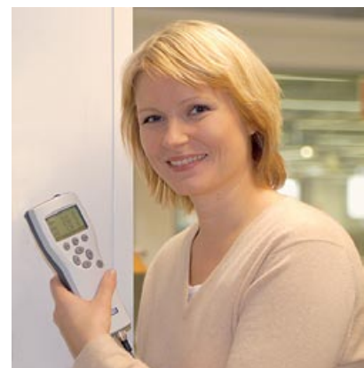
The optional Vaisala MI70 indicator can be used as a display for the DMT152 and for logging data.
