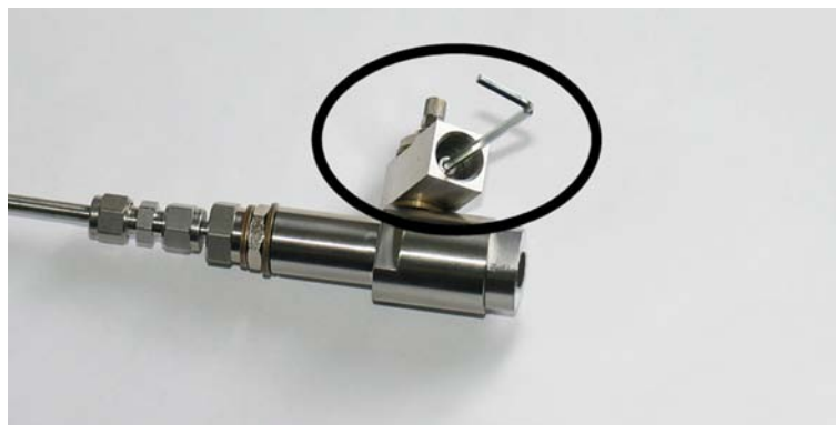
Figure 13 Removing the Leak Screw
