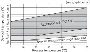
Dewpoint accuracy vs. measurement conditions Response time 63% [90%] at +20 °C gas temperature
