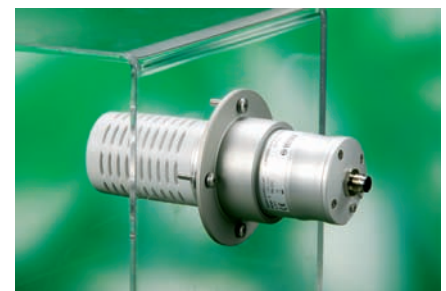
With the optional mounting flange, the GMP343 can for example be installed directly into a soil respiration box. The diffusion-aspirated probe eliminates sampling systems and errors related to pressure differences caused by pumps.
