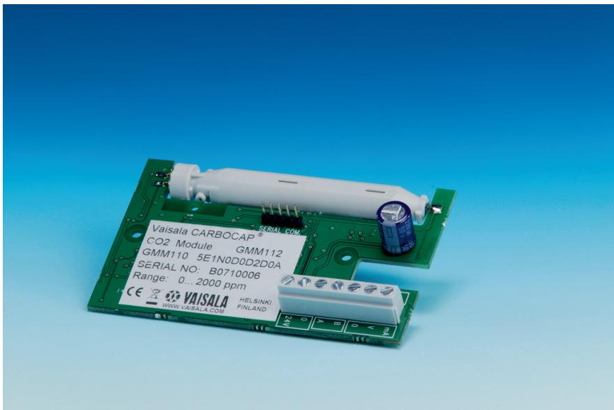
The Vaisala CARBOCAP® Carbon Dioxide Module GMM112 is a basic CO<sub>2</sub> measurement module.
