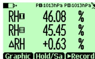
6. Ensure that the probes are located in the same conditions. You can have an optional probe holder for the HMP76 probe to
