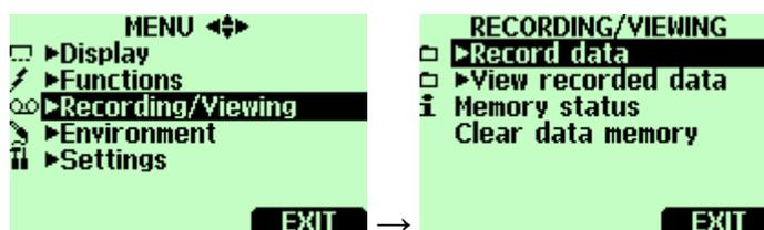
You can record measurement data and view the recorded data on the display.
