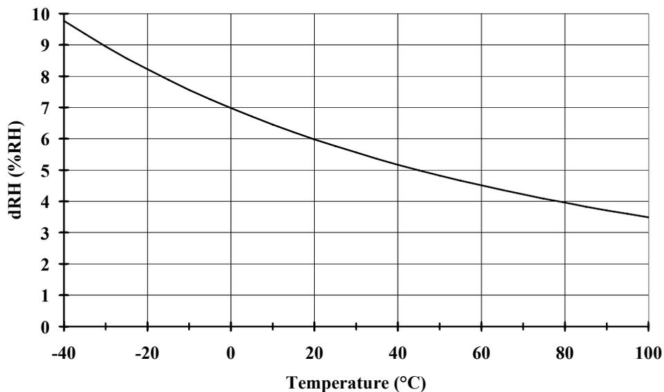
**Measurement error at 100 %RH when the difference between the ambient and sensor temperature is 1 °C.**
