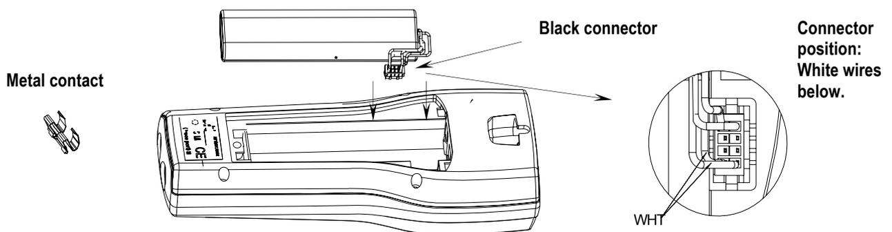
**Installing the battery**
