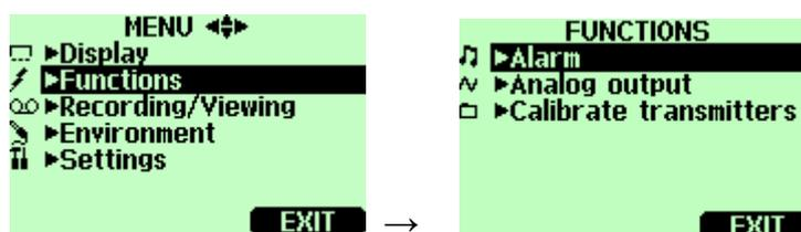
HM70 is alarming by beeping and blinking the backlight. The alarm turns on when the measured value is not between the alarm limits (permissible area). Alarm level(s) can be set for only one quantity at a time. Set the alarm levels as follows:
