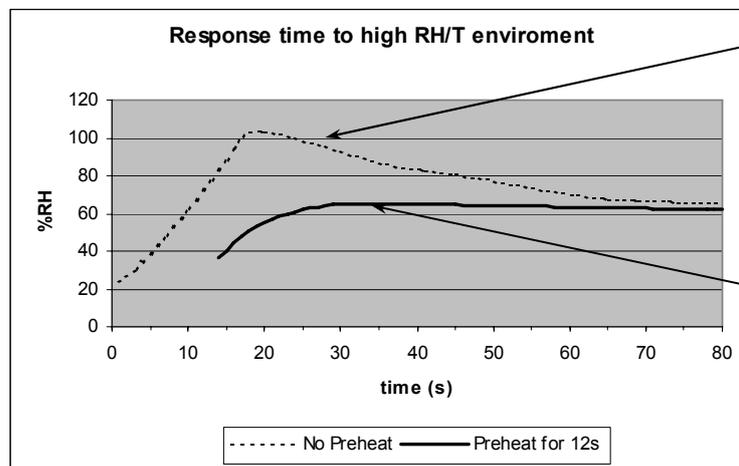
This curve shows how relative humidity increases as a consequence of condensation on the sensor. The correct response is achieved not until the sensor is dried.
