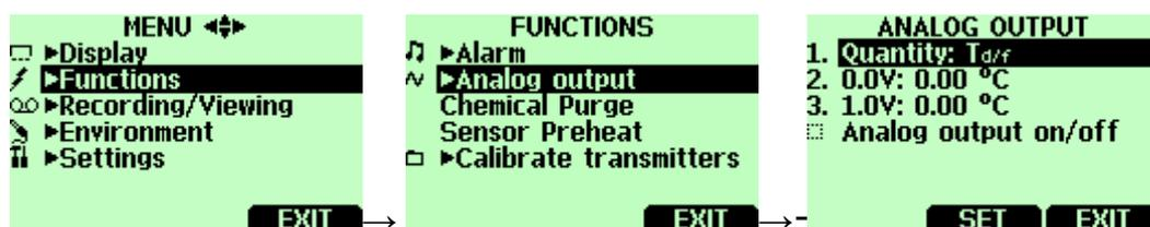
To get analog measurement data, you need the analog output signal cable, see list of accessories on page 73. One voltage signal channel 0...1.0V can be scaled for the selected quantity.
