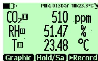
Example of the display when carbon dioxide and humidity probe connected simultaneously to the MI70 indicator.
