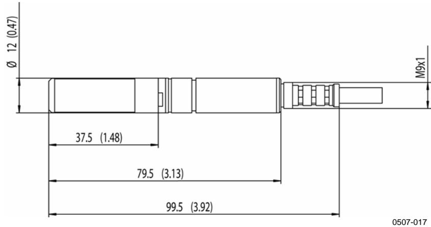
Figure 67 HMT337 Probe Dimensions
