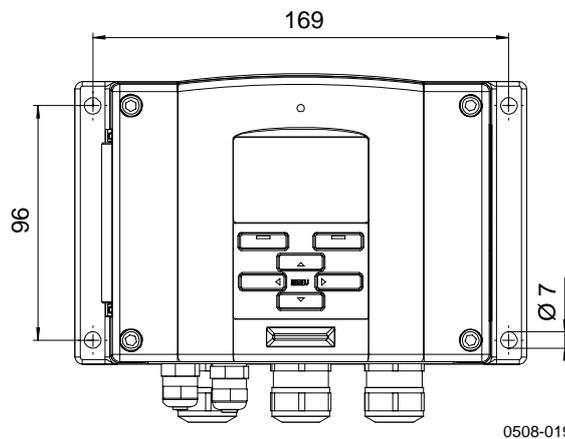
**Figure 4** Standard Mounting
