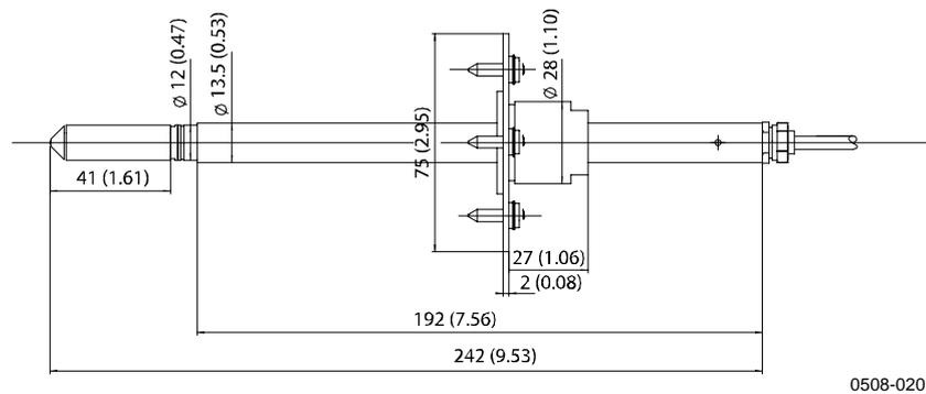
Figure 66 HMT335 Probe Dimensions
