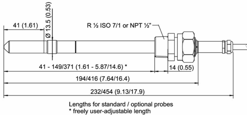
Figure 68 HMT338 Probe Dimensions
