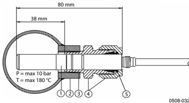
**Figure 72 Swagelok Installation Kit for RH-probe**
