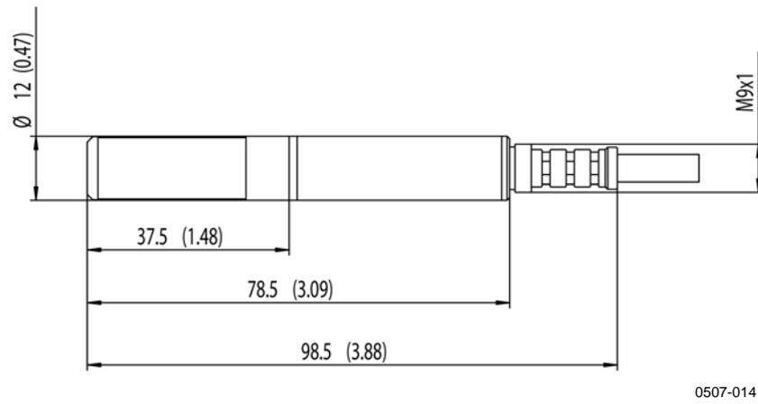
**Figure 64 HMT333 Probe Dimensions**
