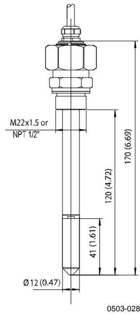
Figure 65 HMT334 Probe Dimensions
