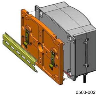
**Figure 7** Mounting with the DIN Rail Installation Kit
