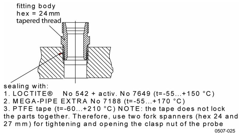
**Figure 26 Sealing of Fitting Body into Process**
