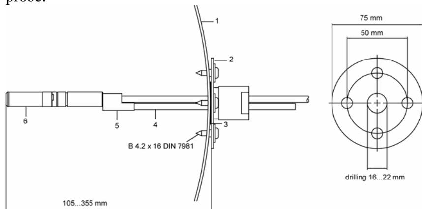
**Figure 70 Duct Mounting Installation Kit**
