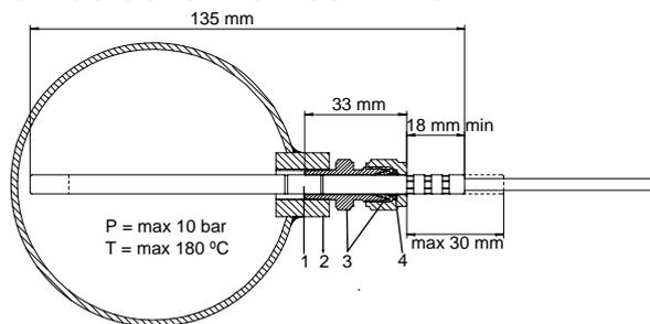
**Figure 73 Swagelok Installation Kit for T-Probe**
