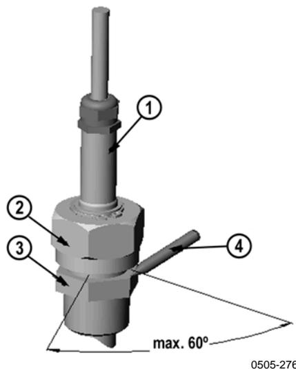
**Figure 27 Tightening the Clasp Nut**
