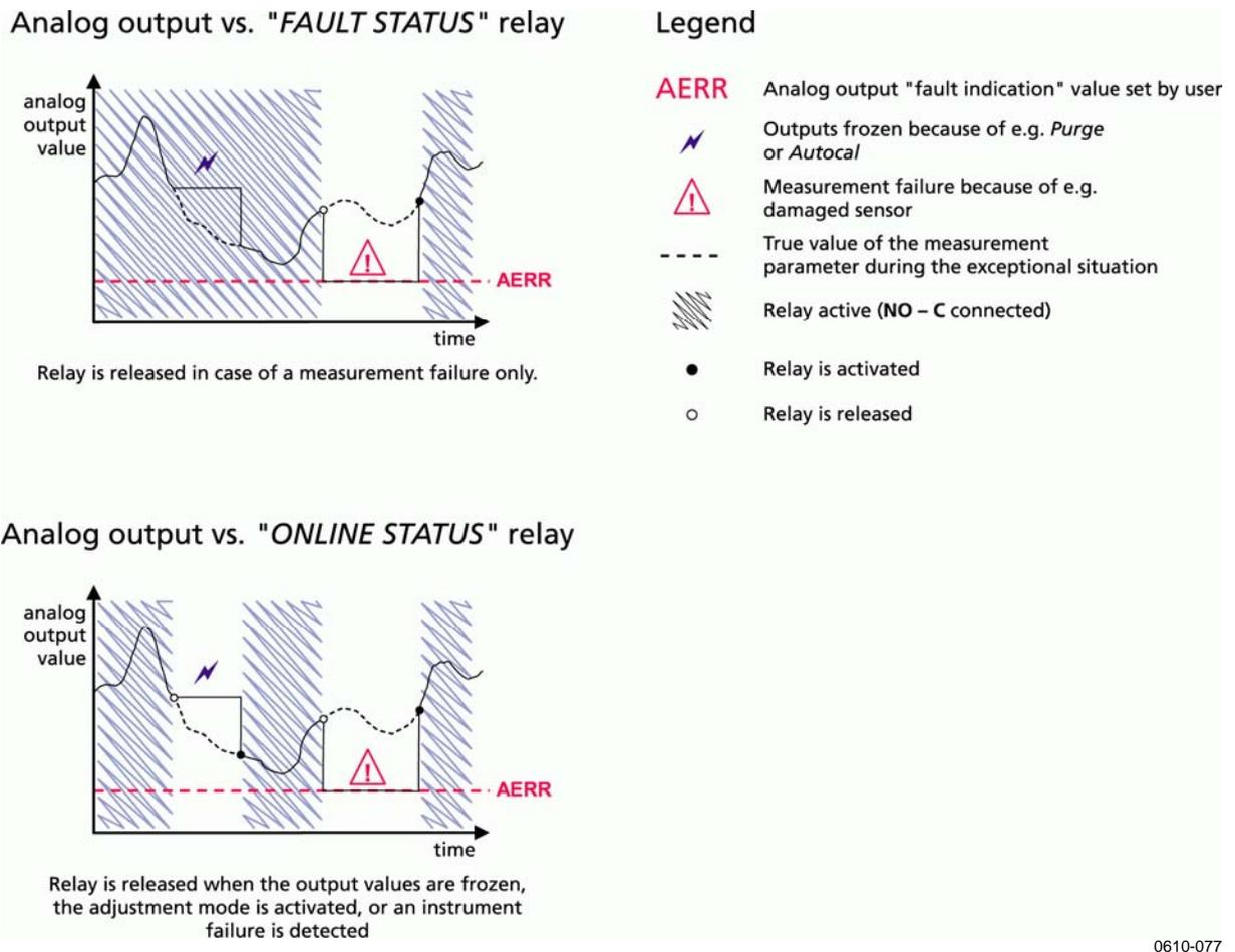
**Figure 49** FAULT/ONLINE STATUS Relay Output Modes
