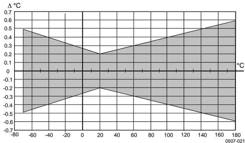
**Figure 60 Accuracy over Temperature Range**
