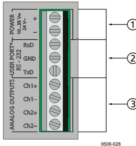
**Figure 17 Screw Terminal Block on Motherboard**
