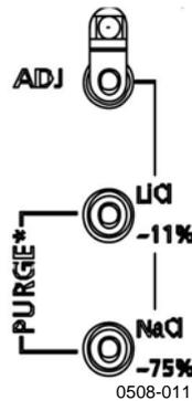
Figure 52 Purge Buttons on Motherboard
