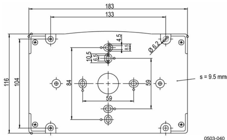
**Figure 6 Dimensions of the Plastic Mounting Plate**
