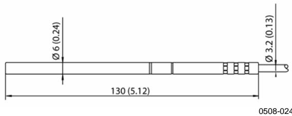
Figure 69 Optional Temperature Probe Dimensions
