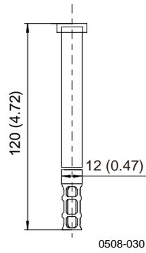
**Figure 63 HMT331 Probe Dimensions**
