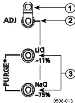
**Figure 57 Adjustment and Purge Buttons**
