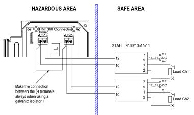
Stahl 9160/13-11-11 Galvanic Isolator Safety factors:  $U_i = 30 V$ ;  $I_i = 100 mA$ ;  $C_i$ ,  $L_i = negligible$
