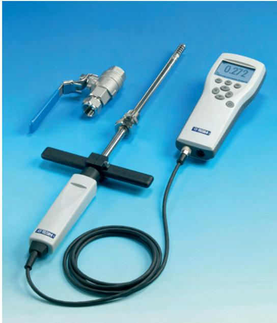
*The MM70 is an ideal tool for the preventive maintenance of oil-filled systems. The water activity measurement indicates the margin to free water formation, which causes severe problems in lubrication systems.*
