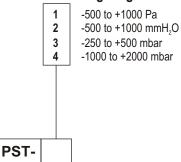
**Example : PST-3** corresponds to a PST manostat with measuring range from -250 to +500 mbar.
