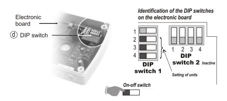
To configure the transmitter, it must not be energized. Then, you can make the settings required, thanks to the DIP switches (as shown on the drawing beside). When the transmitter is configured, you can power it up.
