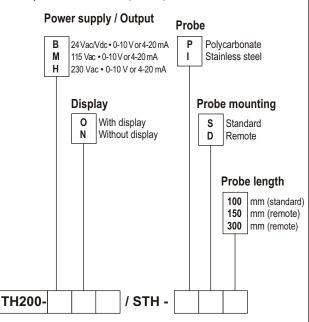
**Example : TH200-BN/STH-PD300 =** humidity transmitter type TH200, with 24Vac/Vdc power supply, without display with polycarbonate remote probe length 300mm
