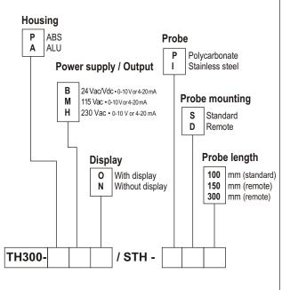
Example: TH300-PBN/STH-PD300 = humidity transmitter type TH300, with ABS housing, 24 Vac/Vdc power supply, without display, with polycarbonate remote probe length 300mm.
